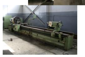
hilst the smaller lathes are perfect for the more intricate turning work and thread cutting on a regular daily basis, the long bed lathe is specifically designed for machining longer than average components. The continuous, single piece bed means that what ever the length of the work piece both ends of the machine are always in line.
