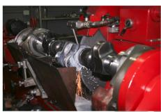
A IM is the only company in Hurghada and the Red Sea area that can offer the very specialized activity of machining and grinding the bearing journals on crankshafts and camshafts from fuel or diesel engines undergoing overhaul.
